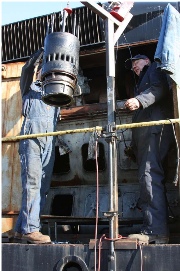
(TOP LEFT) After it's clear of the block, the liner is lowered to the running board and picked up by the hand-rail crane.
