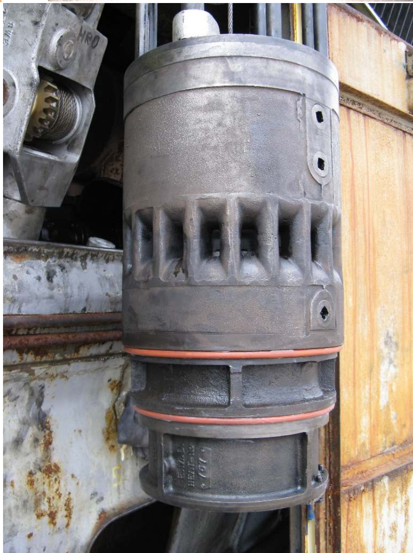
(BOTTOM RIGHT) Here we see one of the 567B liners hanging from the top deck crane, ready to be reinstalled into the engine block after being cleaned and qualified. The two orange O-rings toward the bottom of the liner bracket the water intake for the 567B. These are the gaskets that failed on the 621's engine. The old gaskets came off in multiple pieces. It was no wonder they no longer sealed properly and allowed water to leak in to the crankcase.
