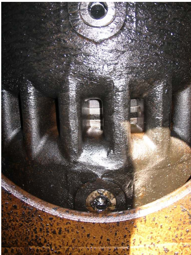
(TOP LEFT) This is looking directly at the side of one of the 567B liners through the air box inspection cover.
