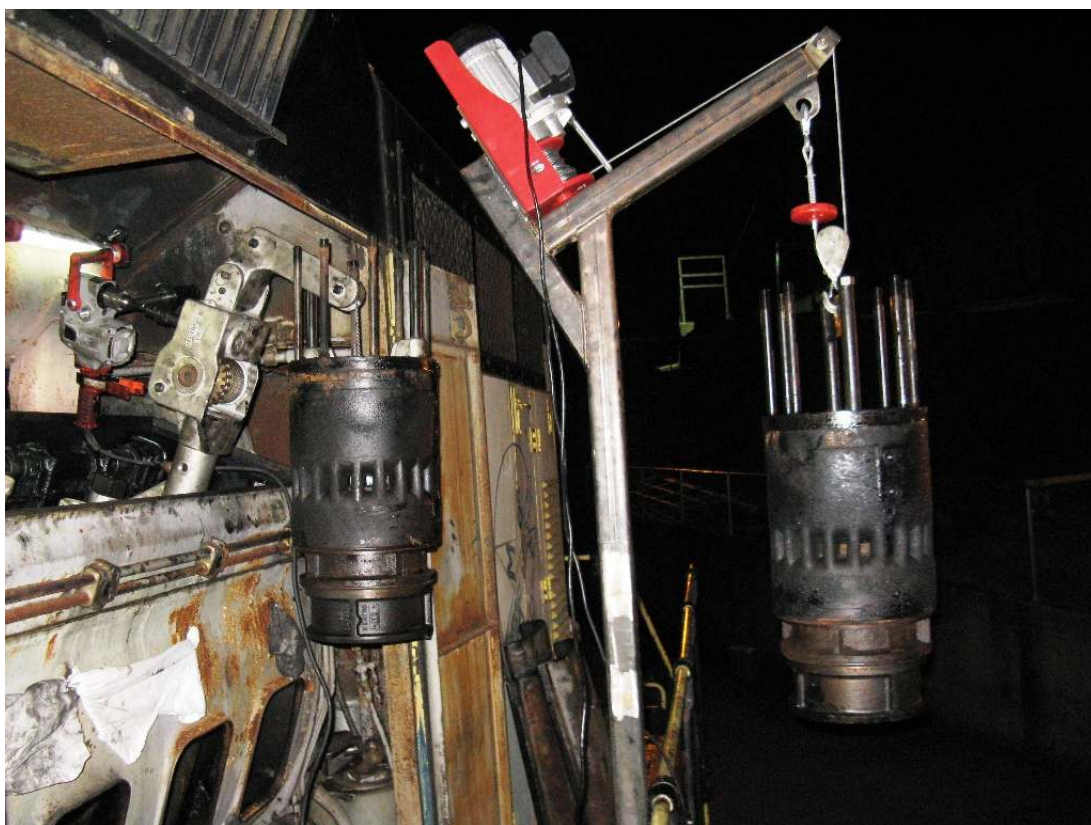
(TOP LEFT) After it's clear of the block, the liner is lowered to the running board and picked up by the hand-rail crane.
